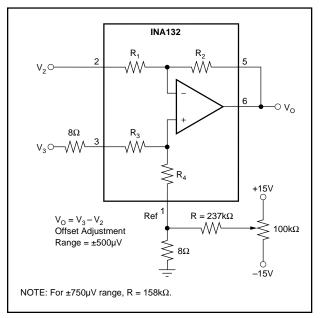
FIGURE 2. Offset Adjustment.
