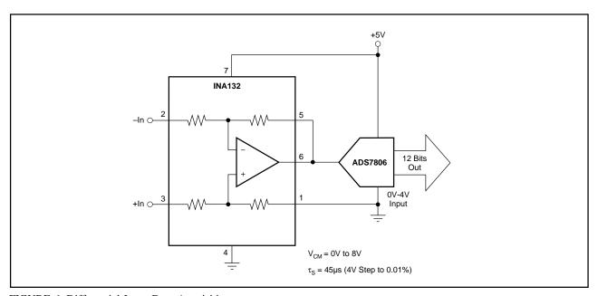
FIGURE 6. Differential Input Data Acquisition.
