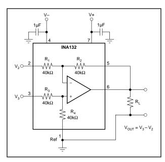
FIGURE 1. Basic Power Supply and Signal Connections.
