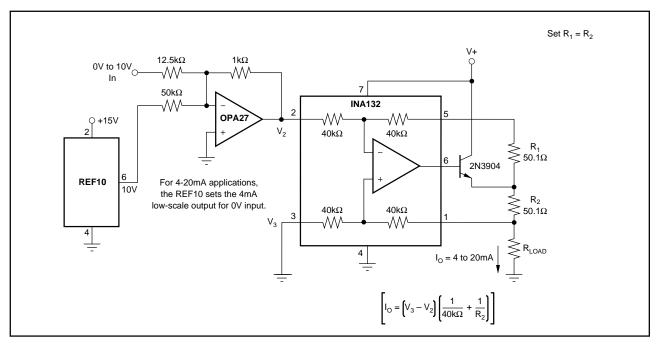
FIGURE 7. Precision Voltage-to-Current Conversion.
