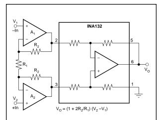
The INA132 can be combined with op amps to form a complete instrumentation amplifier with specialized performance characteristics. Burr-Brown offers many complete high performance IAs. Products with related performances are shown at the right.
