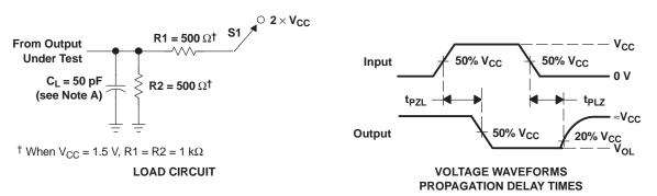
NOTES: A. C<sub>L</sub> includes probe and jig capacitance.
