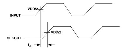
Figure 3. Input to Output Skew
