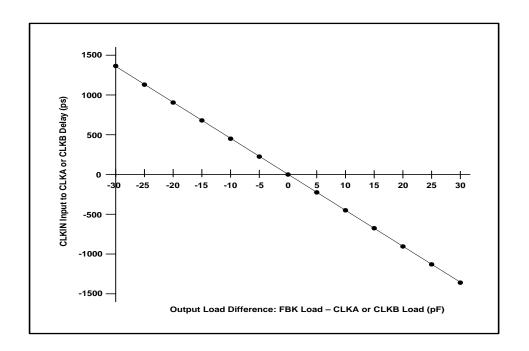
Figure 1. CLKIN Input to CLK A and B Delay (In terms of load difference between CLKOUT and CLK A and B)
