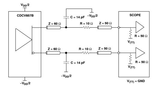
Figure 2. Output Load Test Circuit
