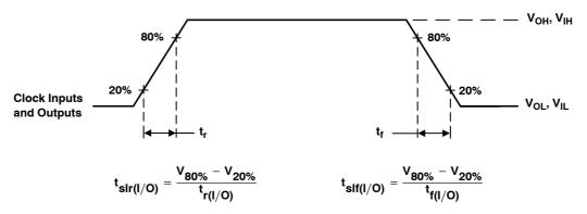
Figure 9. Input and Output Slew Rates
