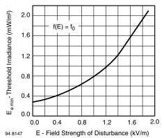
Figure 8. Sensitivity vs. Electric Field Disturbances
