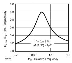
Figure 5. Frequency Dependence of Responsivity
