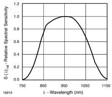
Figure 11. Relative Spectral Sensitivity vs. Wavelength
