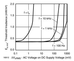
Figure 7. Sensitivity vs. Supply Voltage Disturbances
