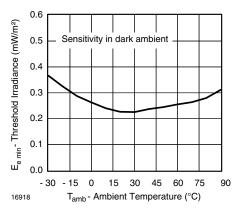
Figure 10. Sensitivity vs. Ambient Temperature
