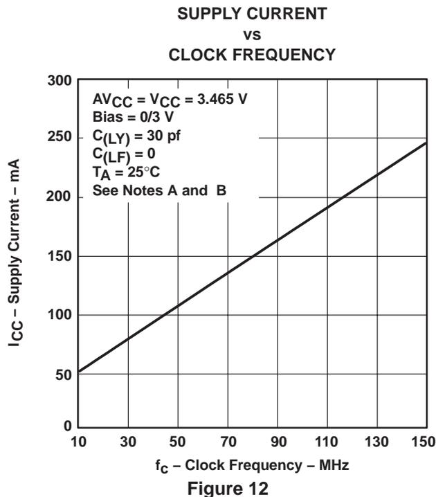
NOTES: A.  $C_{(LY)}$  = Lumped capacitive load at Y
