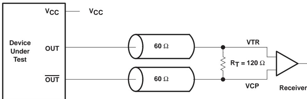
Figure 3. Differential Signal Using Direct Termination Resistor
