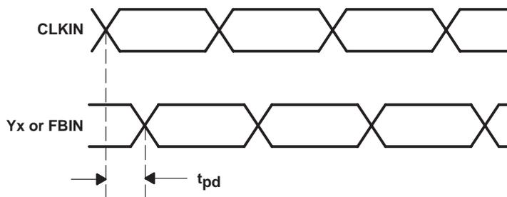
Figure 5. Propagation Delay Time;  $t_{pLH}$ ,  $t_{pHL}$
