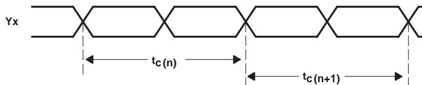
NOTE A: Cycle-to-cycle jitter =  $|t_{c(n)} - t_{c(n+1)}|$  over 2000 consecutive cycles.
