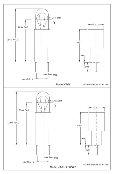
Mounting: Printed circuit Board Mounting pattern on page SP2. Terminals: Tinned brass Housing: White nylon Lamp: T-1 3/4 Wedge base
