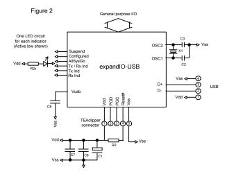
Oscillator X1/C2/C3 may be replaced by a low-cost resonator, provided its frequency tolerance is greater than 0.25% (full speed devices) or 1.5% (low speed devices). C1 and C6 should be placed close to the USB connector. Capacitor(s) C7 should be placed near the Vss and Vdd pin(s) of the expandIO-USB and are only required if they would be some distance from C6. C8 is a filter capacitor for an internal regulator and is required.
