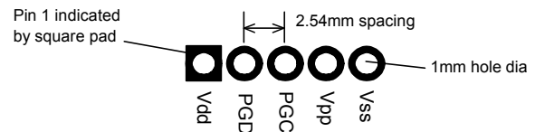
Figure 13. Recommended plate-through connector design
