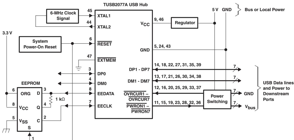
Figure 6. Typical Application of the TUSB2077A USB Hub
