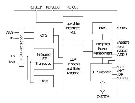
Figure 1 USB3310 Block Diagram
