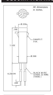
Mounting: Ø.310 MIN. hole in panels .020/.062 thick, use speednut #SN1287 for other panel thickness.
