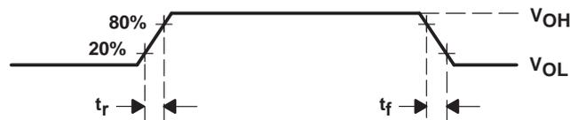
Figure 7. Voltage Waveforms
