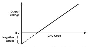
Figure 14. Effect of Negative Offset (single supply)
