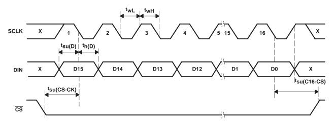
Figure 1. Timing Diagram
