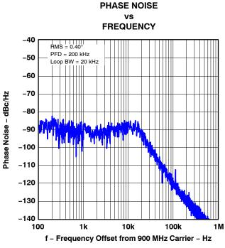
Figure 12. Integrated Phase Noise (RFOUT = 900 MHz)
