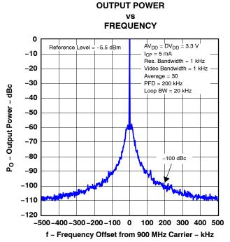
Figure 10. Reference Spurs (RFOUT = 900 MHz)
