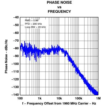
Figure 17. Integrated Phase Noise (RFOUT = 1960 MHz)
