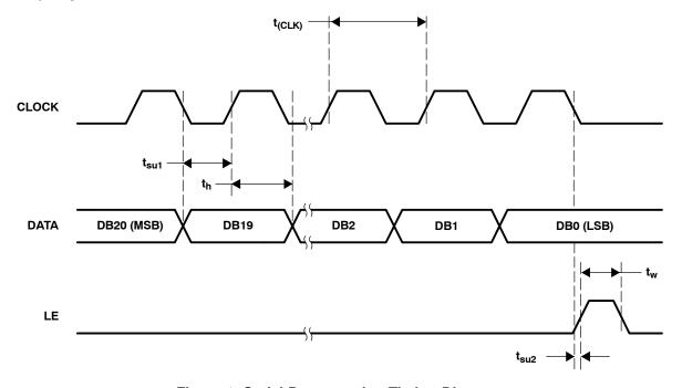
Figure 1. Serial Programming Timing Diagram
