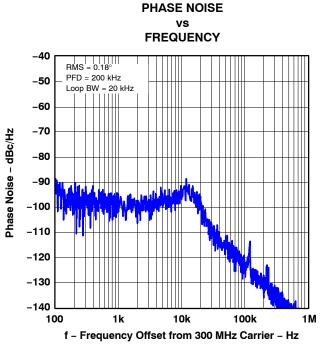
Figure 5. Integrated Phase Noise (RFOUT = 300 MHz)
