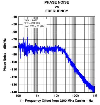
Figure 19. Integrated Phase Noise (RFOUT = 2200 MHz)
