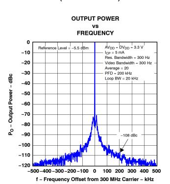
Figure 4. Reference Spurs (RFOUT = 300 MHz)
