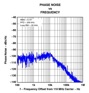
Figure 3. Integrated Phase Noise (RFOUT = 110 MHz)
