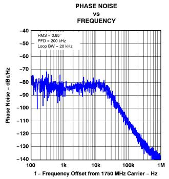
Figure 14. Phase Noise (RFOUT = 1750 MHz)
