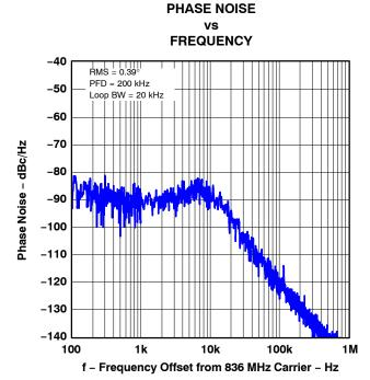
Figure 9. Integrated Phase Noise (RFOUT = 836 MHz)
