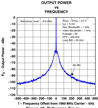
Figure 15. Reference Spurs (RFOUT = 1960 MHz)
