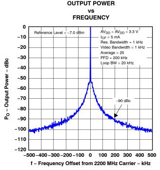
Figure 18. Reference Spurs (RFOUT = 2200 MHz)
