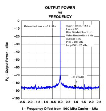
Figure 16. Phase Noise (RFOUT = 1960 MHz)
