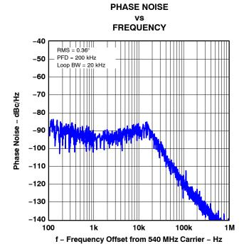
Figure 7. Integrated Phase Noise (RFOUT = 540 MHz)
