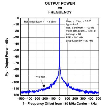
Figure 2. Reference Spurs (RFOUT = 110 MHz)
