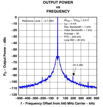
Figure 6. Reference Spurs (RFOUT = 540 MHz)
