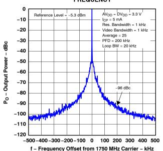
Figure 13. Reference Spurs (RFOUT = 1750 MHz)
