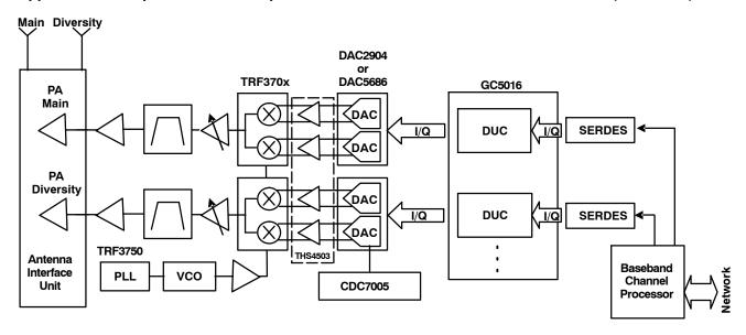
Figure 27. Texas Instruments' Proposed Direct Upconversion Wireless Infrastructure Transmitter Architecture
