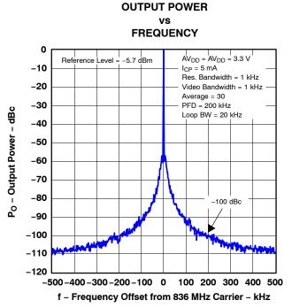
Figure 8. Reference Spurs (RFOUT = 836 MHz)
