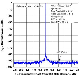
Figure 11. Phase Noise (RFOUT = 900 MHz)
