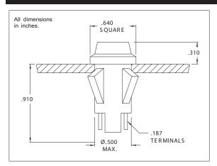
Mounting: Will snap-fit into Ø.500/.505 hole in panels .020/.100 thick. Push-on speednut SN0461 also available.
