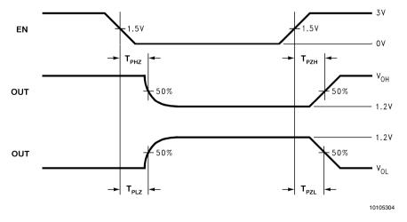
FIGURE 3. Output active to TRI-STATE and TRI-STATE to active output time
