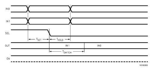
FIGURE 2. Input-to-Select falling edge setup and hold times and mux switch time
