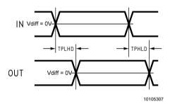
FIGURE 6. Propagation Delay Low-to-High and High-to-Low
