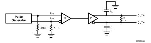
FIGURE 4. LVDS Output Load
