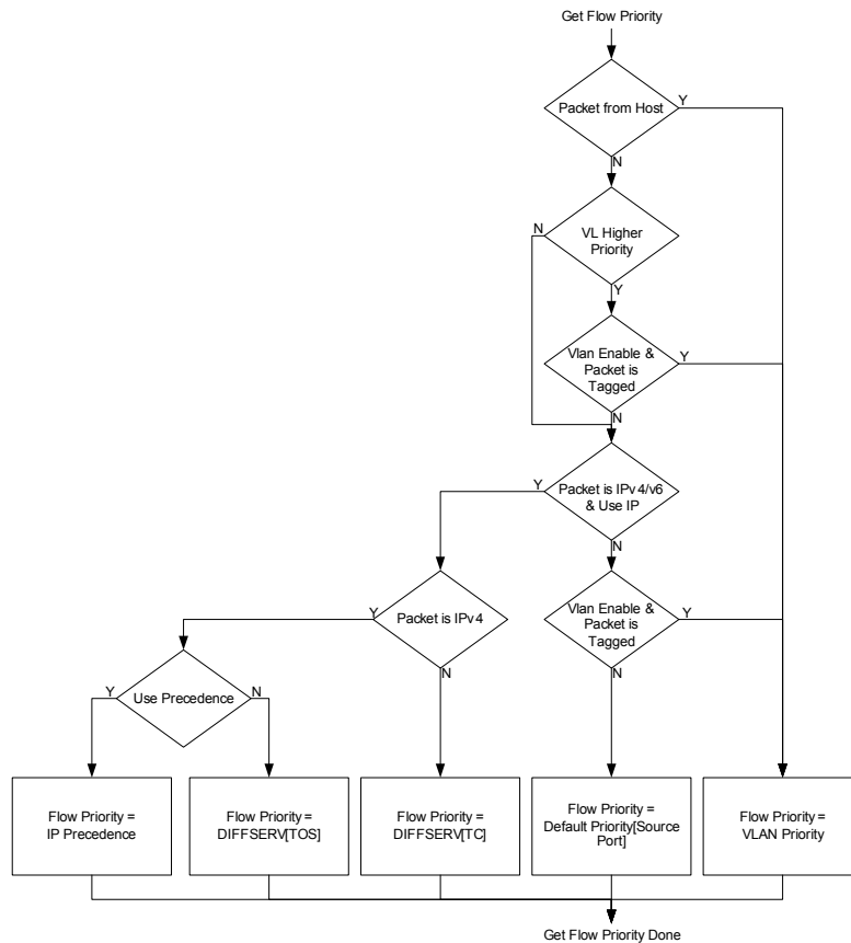
Figure 6.8 Switch Engine Ingress Flow Priority Calculation
