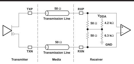
Figure 24. High-Speed I/O Directly-Coupled Mode
