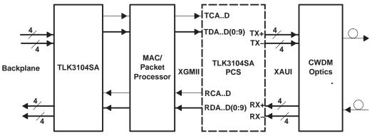
Figure 2. System Block Diagram (PCS Implementation)
