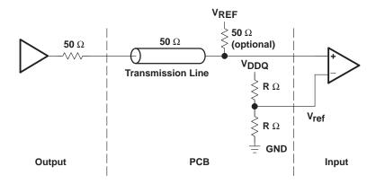
NOTE: The output buffer of the TLK3104SA has on-chip termination of 50  $\Omega$ . The output signal is compliant with the JEDEC SSTL\_2 Class 1 specification. Line termination on the receive end is optional and not recommended for low-power applications.
