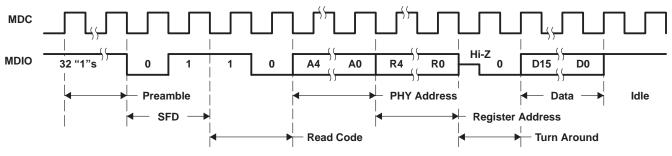
Figure 15. Management Interface Read Timing
