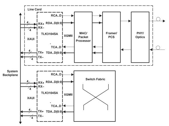
Figure 3. System Block Diagram (Backplane Interconnect Implementation)
