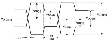
Figure 17. Differential and Common-Mode Output Voltage Definitions
