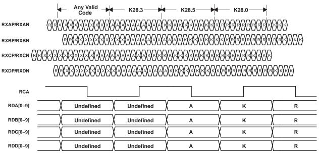
Figure 12. Channel Synchronization Using Alignment Code
