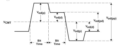
Figure 14. Output Differential Voltage Under Preemphasis
