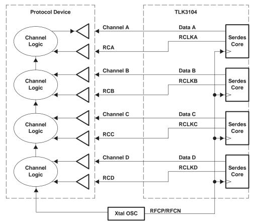
Figure 13. Receive and Reference Clock Relationship (Independent Channel Modes)
