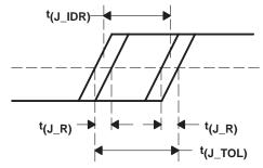
NOTE:  $t_{(J_TOL)} = t_{(J_R)} + t_{(J_IDR)}$ , where  $t_{(J_TOL)}$  is the receive jitter tolerance,  $t_{(J_IDR)}$  is the received deterministic jitter, and  $t_{(J_R)}$  is the Gaussian random edge jitter distribution at a maximum BER = 10<sup>-12</sup>.
