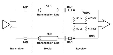
Figure 25. Example High-Speed I/O AC-Coupled Mode
