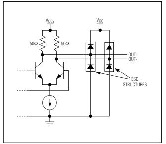
Figure 1. CML Output Structure
