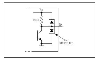
Figure 4. Signal-Detect Output Circuit
