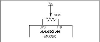
Figure 3. Connecting a Potentionmeter Across HFPD and LFPD
