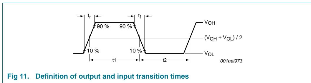
**Fig 11. Definition of output and input transition times**
