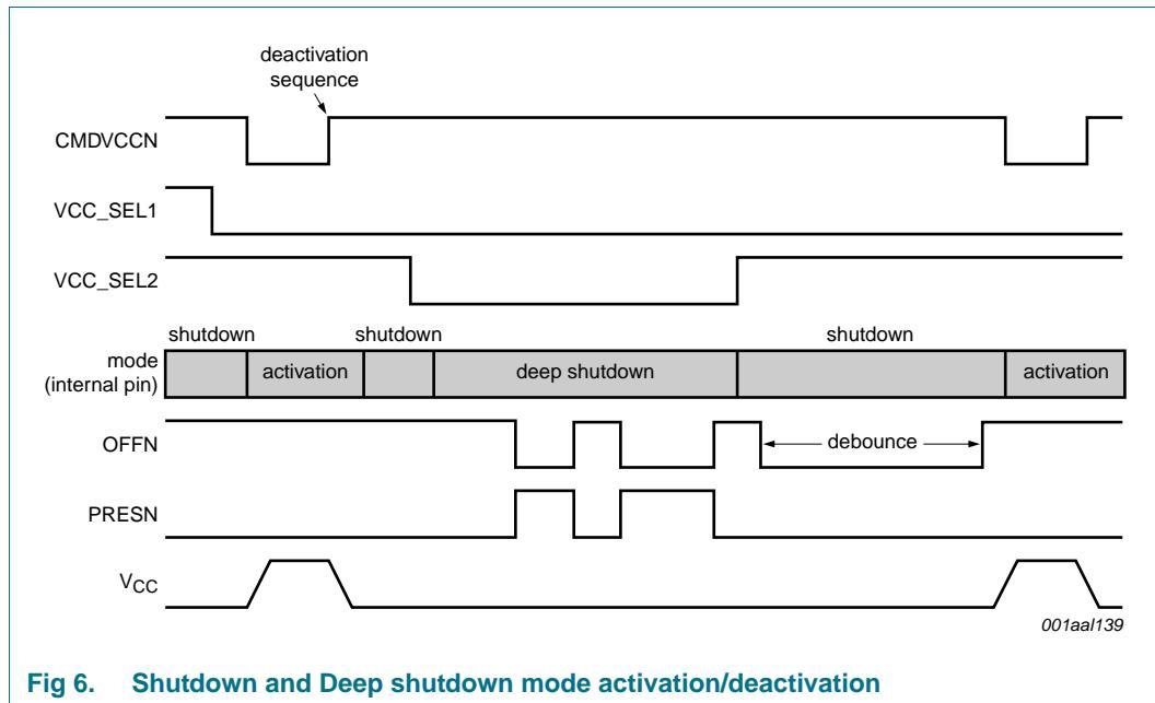
Fig 6. Shutdown and Deep shutdown mode activation/deactivation
