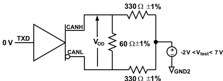
Figure 3. Driver VOD with Common-mode Loading Test Circuit
