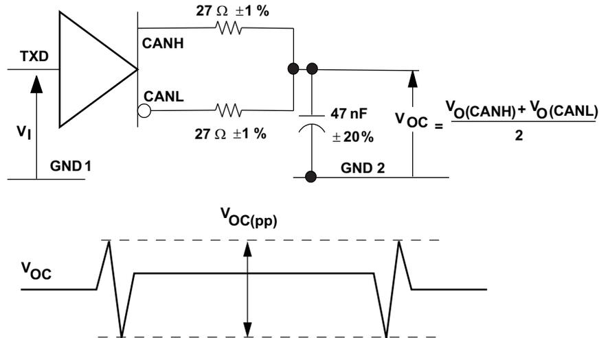
Figure 8. Peak-to-Peak Output Voltage Test Circuit and Waveform
