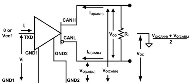
Figure 1. Driver Voltage, Current and Test Definitions
