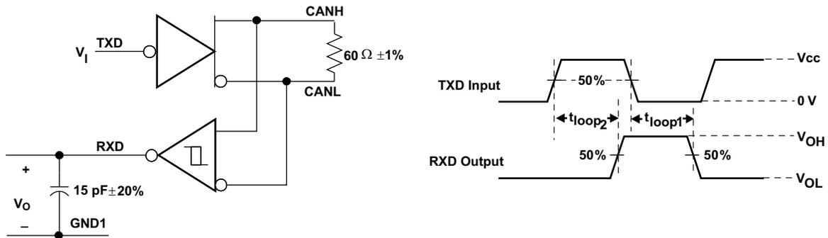
Figure 9.  $t_{LOOP}$  Test Circuit and Voltage Waveforms
