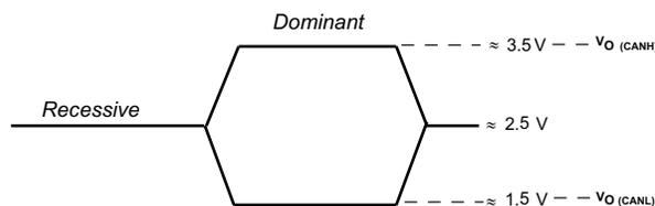
Figure 2. Bus Logic State Voltage Definitions
