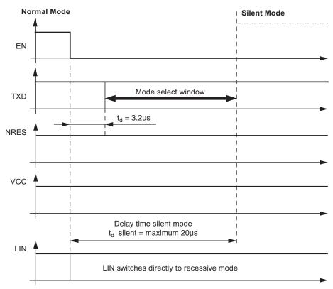
Figure 4-2. Switch to Silent Mode
