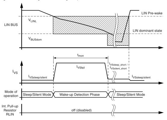
Figure 4-6. Floating LIN-bus During Sleep or Silent Mode
