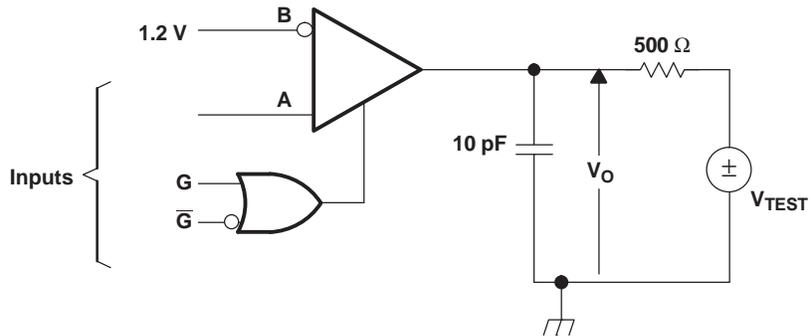
NOTE: All input pulses are supplied by a generator having the following characteristics:  $t_r$  or  $t_f \leq 1$  ns, pulse repetition rate (PRR) = 0.5 Mpps, pulsewidth =  $500 \pm 10$  ns.  $C_L$  includes instrumentation and fixture capacitance within 0,06 mm of the D.U.T.
