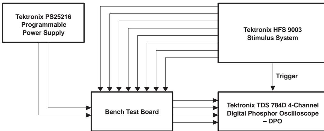
**Figure 16. Equipment Setup**
