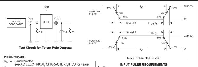
Load capacitance includes jig and probe capacitance; see AC ELECTRICAL CHARACTERISTICS for value. Termination resistance should be equal to  $Z_{OUT}$  of
