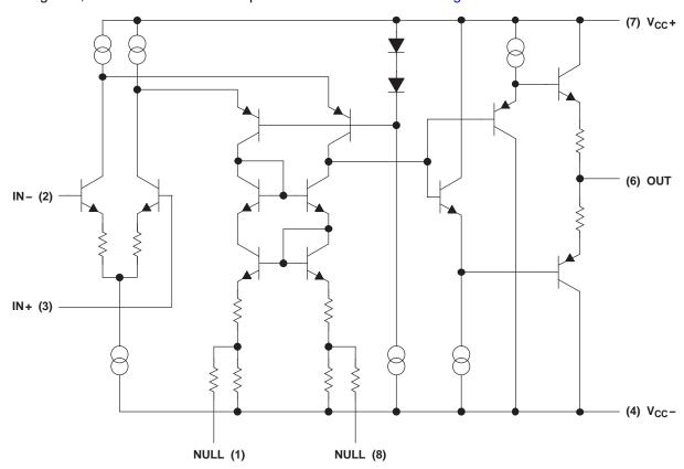
Figure 51. THS4031 Simplified Schematic
