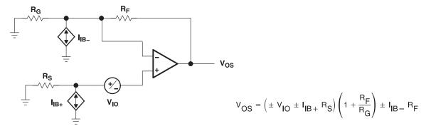
Figure 57. Output Offset Voltage Model
