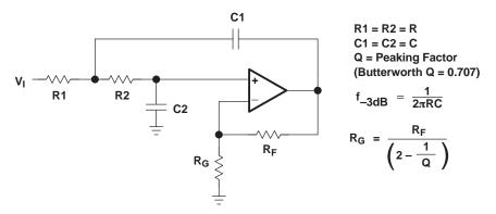
Figure 59. Two-Pole Low-Pass Sallen-Key Filter
