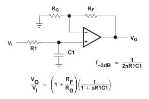
Figure 58. Single-Pole Low-Pass Filter
