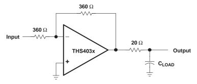
Figure 55. Driving a Capacitive Load
