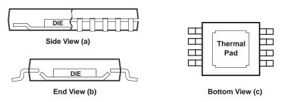
A. The thermal pad is electrically isolated from all terminals in the package.
