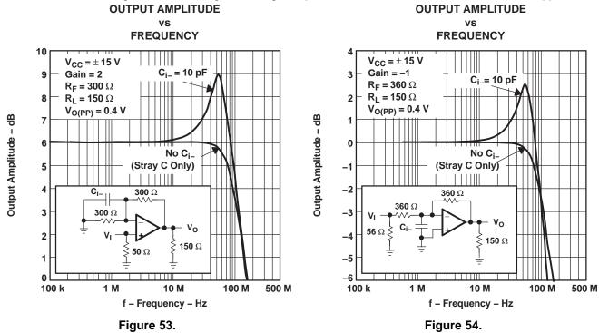
The second precaution to help maintain a smooth frequency response is to keep the feedback resistor  $(R_f)$  and the gain resistor  $(R_g)$  values fairly low. These two resistors are effectively in parallel when looking at the ac small-signal response. But, as can be seen in Figure 26 through Figure 37, a value too low starts to reduce the bandwidth of the amplifier. Table 1 shows some recommended feedback resistors to be used with the THS403x.
