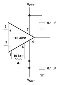
Figure 56. Offset Nulling Schematic
