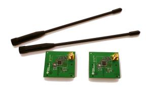
2 x CC1120 or CC1121 Evaluation Modules 2 x Antennas (type depending on frequency)
