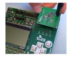
The latter can be used as a carrier board for the Insert a CC112xEM into the TrxEB. The connectors will only fit in one position so that the EM cannot be inserted the wrong way. Do not use excessive force on the EM. Remember to mount the antenna.
