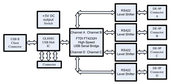
Figure 1.6 - USB2-H-6004/6008/6016-M Main Board Block Diagram
