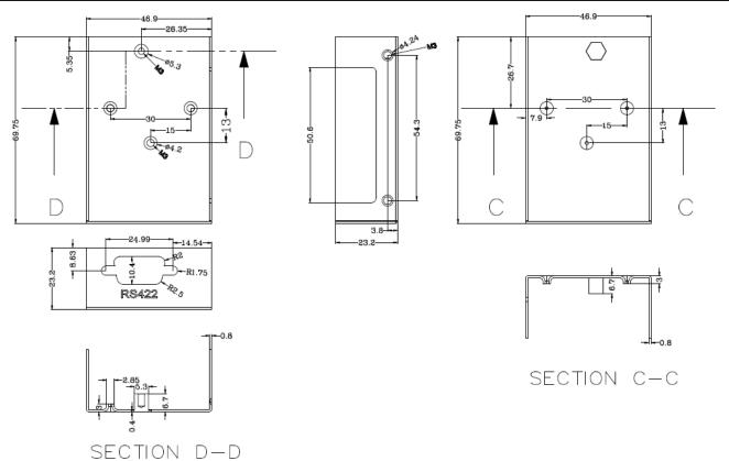
Figure 7.2 - USB2-H-6001-M Bottom Cover of Dimension
