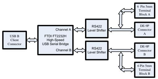
Figure 1.5 - USB2-H-6002-M Block Diagram
