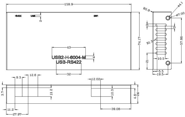
Figure 7.5 - USB2-H-6004-M Top Cover of Dimension
