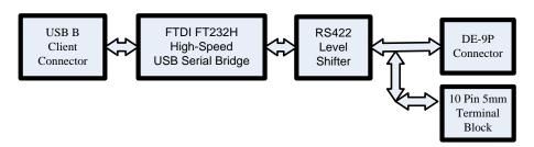
Figure 1.4 - USB2-H-6001-M Block Diagram
