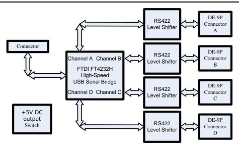
Figure 1.7 - USB2-H-6008/6016-M Daughter Board Block Diagram
