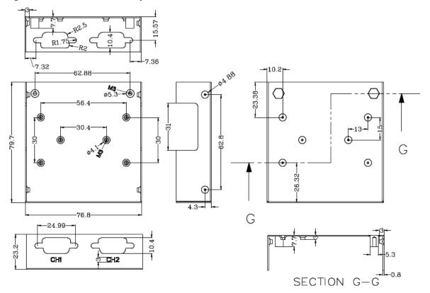
Figure 7.4 - USB2-H-6002-M Bottom Cover of Dimension
