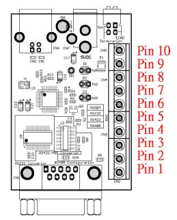
Figure 3.1 - USB2-H-6001-M Terminal Block Connector Assignment
