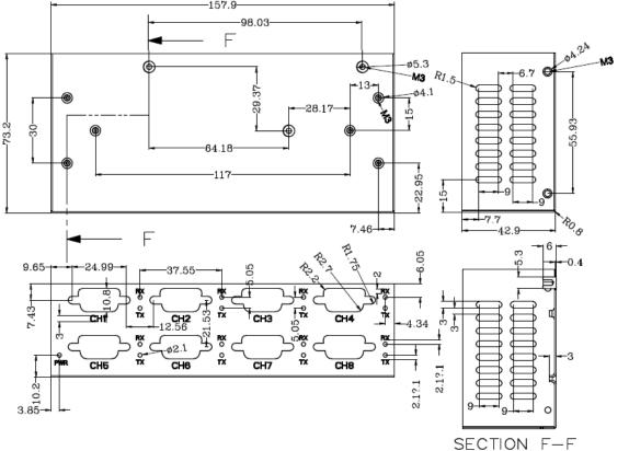
Figure 7.8 - USB2-H-6008-M Bottom Cover of Dimension
