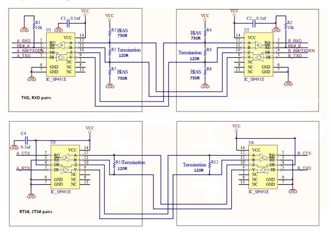
Figure 4.2 - RS422 Network with terminations
