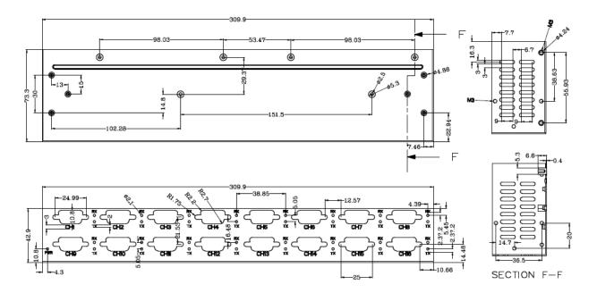
Figure 7.10 - USB2-H-6016-M Bottom Cover of Dimension
