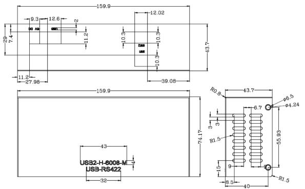
Figure 7.7 - USB2-H-6008-M Top Cover of Dimension
