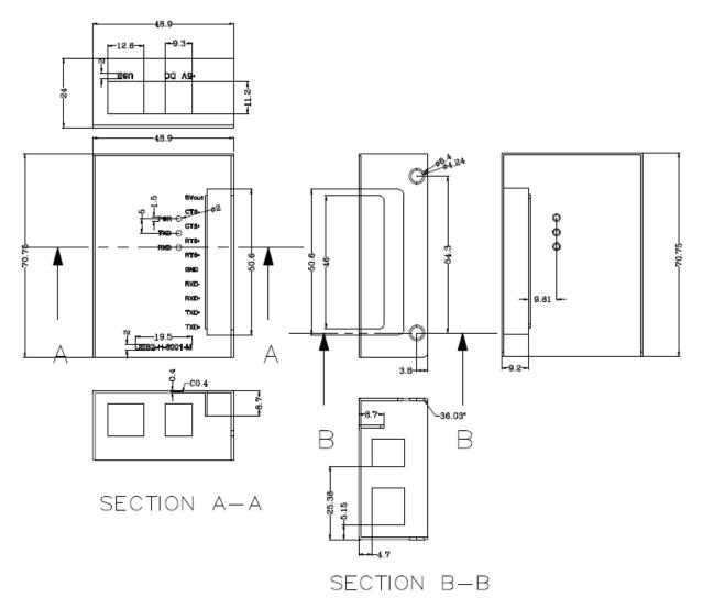
Figure 7.1 - USB2-H-6001-M Top Cover of Dimension
