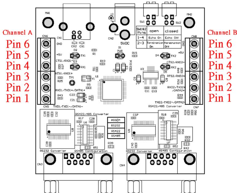
**Figure 3.2 - USB2-H-6002-M Terminal Block Connector Assignment**
