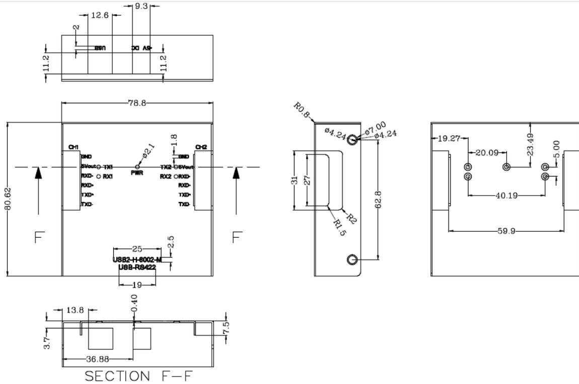
Figure 7.3 - USB2-H-6002-M Top Cover of Dimension
