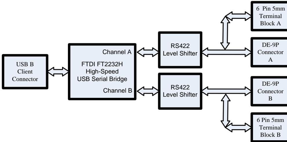
Figure 1.5 - USB2-H-6002-M Block Diagram
