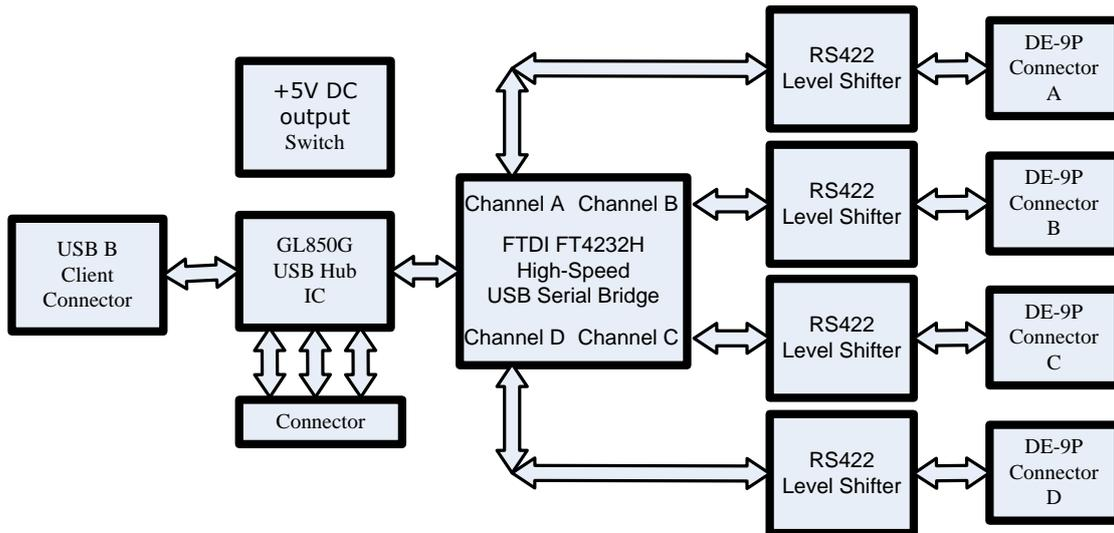
Figure 1.6 - USB2-H-6004/6008/6016-M Main Board Block Diagram
