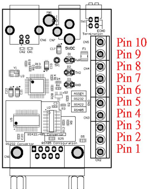
**Figure 3.1 - USB2-H-6001-M Terminal Block Connector Assignment**
