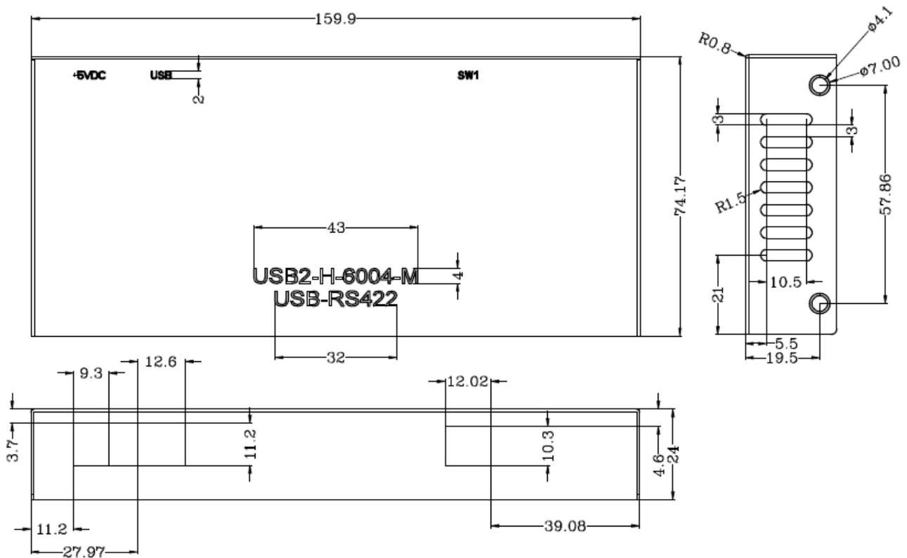
Figure 7.5 - USB2-H-6004-M Top Cover of Dimension
