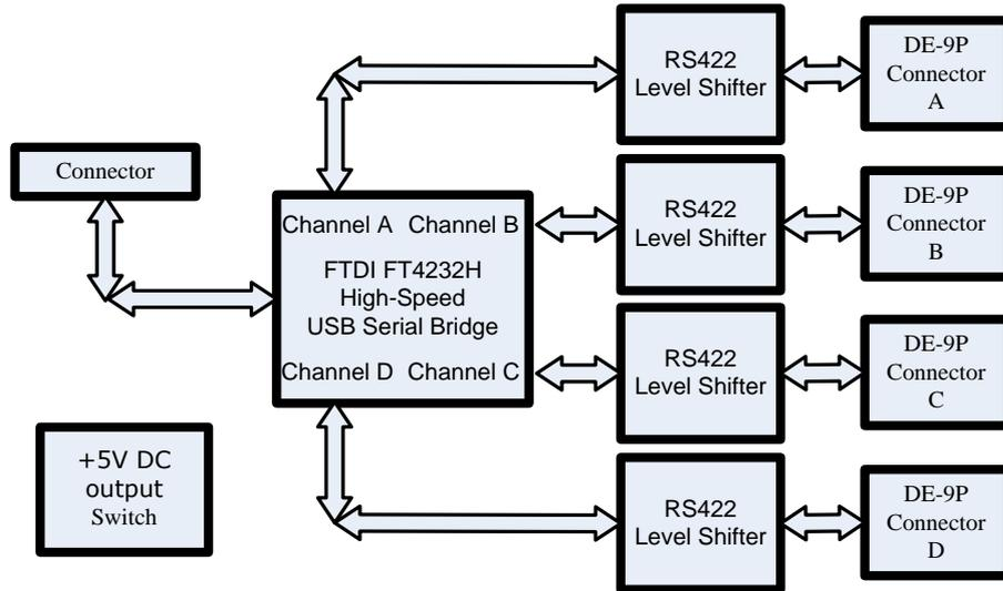
**Figure 1.7 - USB2-H-6008/6016-M Daughter Board Block Diagram**
