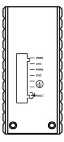
While only one power source is required to power up the media converter, two power sources offer redundancy for those mission critical applications. (PWR1 and PWR2)
