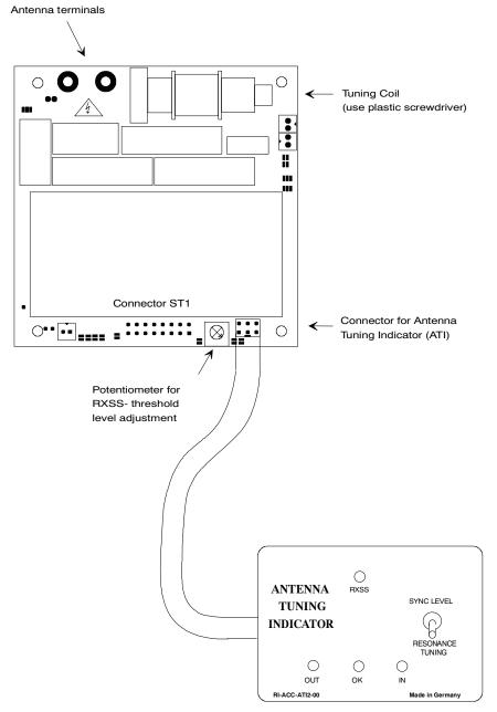
Figure 2-1. Top View of the ATI Connected to the RFM
