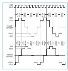
Figure 5: Half Step mode: MS1=1, MS2=0, DIR=1
