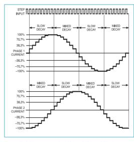
Figure 7: 8 Microstep mode: MS1=1, MS2=1, DIR=1
