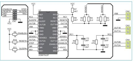
features two independent coils (A and B). Their ending terminals should be connected to the CN3 and CN4 connectors (OUT1A, OUT1B, OUT2A and OUT2B pins). A voltage used for driving these coils is supplied on the CN2 connector and amounts to up to 30V.
