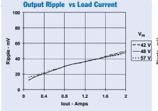
**Output Ripple vs Load Current** 100 80 VIN Ripple - mV 60 --42 V -48 V 57 V 20 0 0.8 0 0.2 0.4 0.6 lout - Amps
