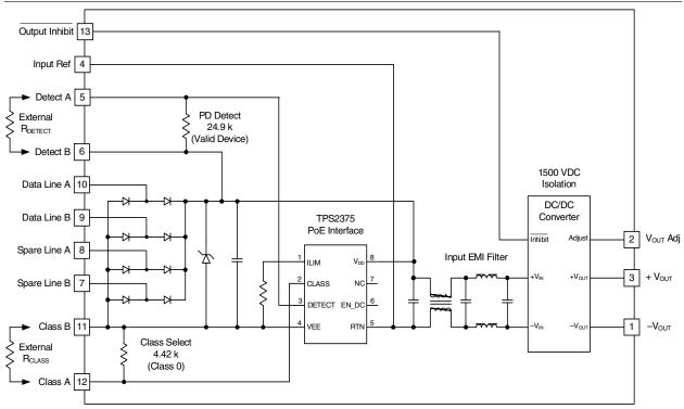
Figure 1 1; Block Diagram of the PTB48540 Series Modules
