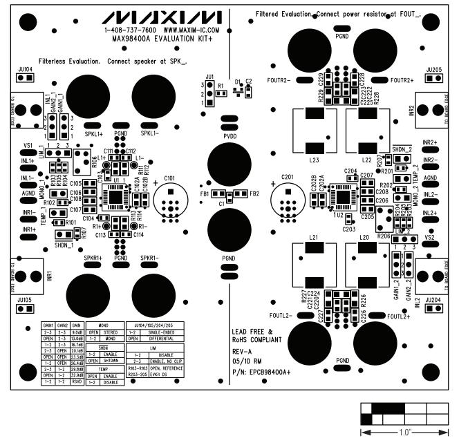
Figure 2. MAX98400A EV Kit Component Placement Guide—Component Side
