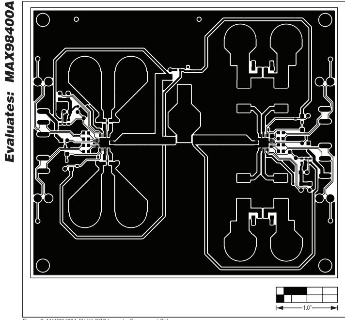
Figure 3. MAX98400A EV Kit PCB Layout—Component Side
