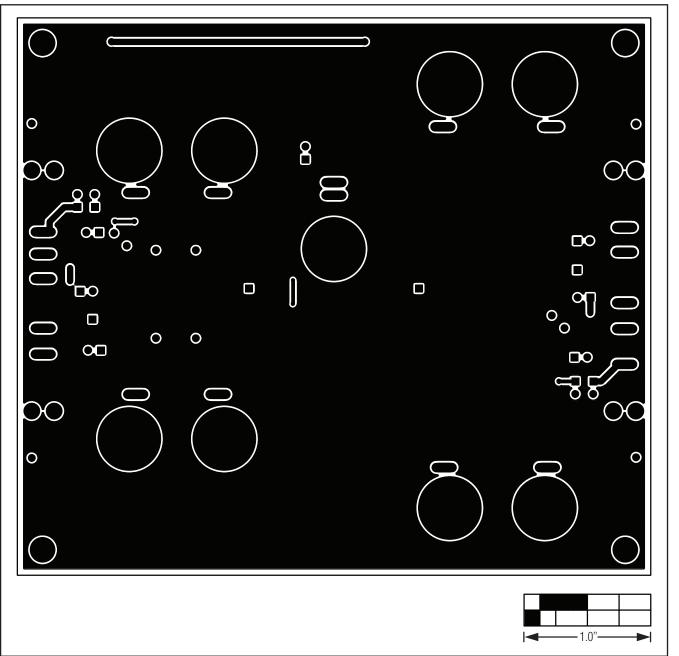
Figure 4. MAX98400A EV Kit PCB Layout—Solder Side
