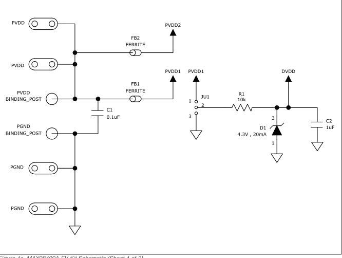
Figure 1a. MAX98400A EV Kit Schematic (Sheet 1 of 3)
