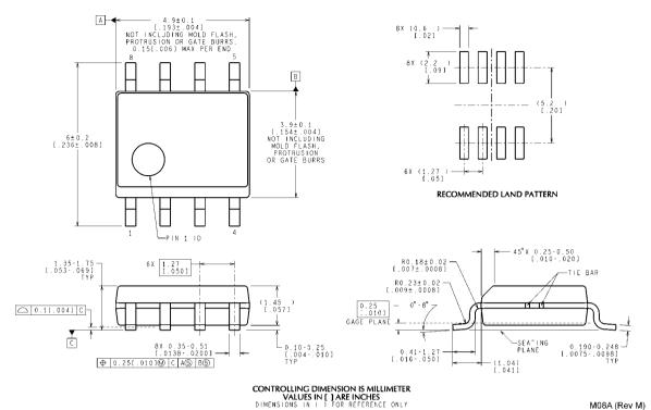
Narrow SOIC Package Order Number LM4562MA NS Package Number M08A
