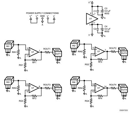
FIGURE 1. Board Schematic
