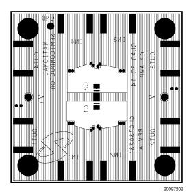
FIGURE 2. Board Layout (Actual size = 2" x 2")
