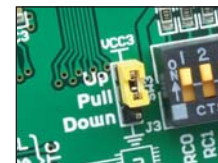
Figure 9-3: J3 in pull-up position
