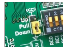
Figure 9-2: J3 in pull-down position
