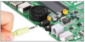
Figure 16-2: 3.5mm connectors CN22 and CN23
