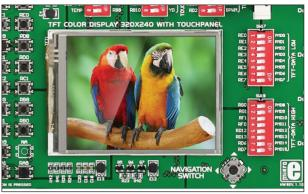
Figure 18-1: TFT display with touch panel
