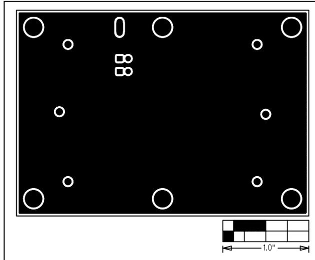
Figure 4. MAX9654 EV Kit PCB Layout—Solder Side
