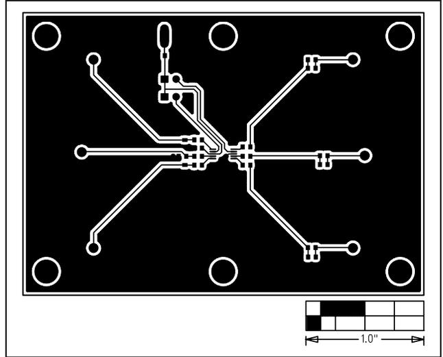
Figure 3. MAX9654 EV Kit PCB Layout—Component Side
