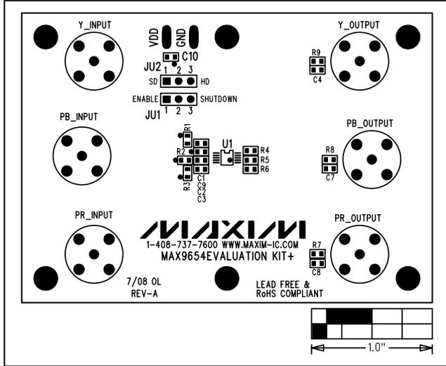
Figure 2. MAX9654 EV Kit Component Placement Guide—Component Side
