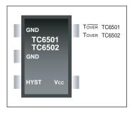
Low cost temperature sensing devices such as the TC6501 and TC6502 (offered in SOT-23 packages) can be conveniently placed near power LED(s) to obtain a more accurate temperature monitoring and provide a logic output fault signal.
