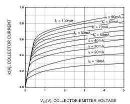
Figure 1. Static Characteristic
