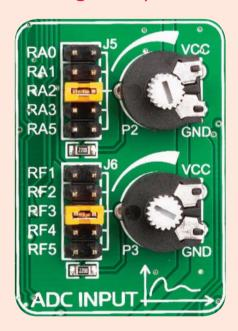
Figure 18-1: use J5 and J6 jumpers to connect analog input lines with potentiometers P2 and P3
