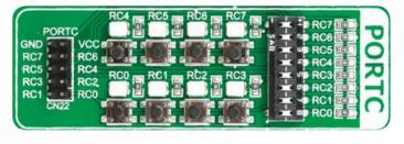
Figure 6-1: I/O group contains 3 PORT headers, tri-state pull up/down DIP switch, buttons and LEDs all in one place
