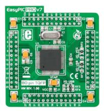
Figure 4-2: Standard 80-pin MCU card with PIC18F87J50, which supports USB.
