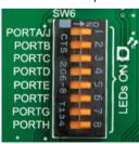
Figure 6-6: SW6.1 through SW6.4 switches are used to enable PORT LEDs
