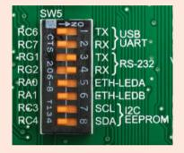
In order to enable RS-232 communication, you must push SW5.3 (RG1) and SW5.4 (RG2) to ON position. This connects the RX and TX lines to appropriate microcontroller pins and its second UART module.
