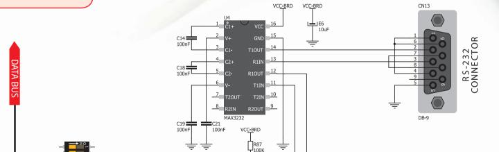
Figure 8-1: RS-232 connection schematics
