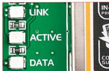
Three LEDs indicate specific programmer operation. **Link** LED lights up when USB link is established with your PC, **Active** LED lights up when programmer is active. **Data** is on when data is being transfered between the programmer and PC software (compiler or mikroProg Suite<sup>™</sup> for PIC<sup>®</sup>).
