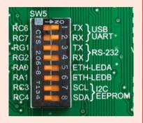
In order to enable USB-UART communication, you must push **SW5.1** (RC6) and **SW5.2** (RC7) to **ON** position. This connects the **RX** and **TX** lines to appropriate microcontroller pins and its first UART module.
