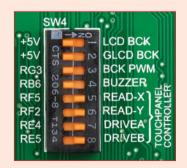
Figure 14-5: Turn on switches 5 through 8 on SW4 to enable Touch panel controller
