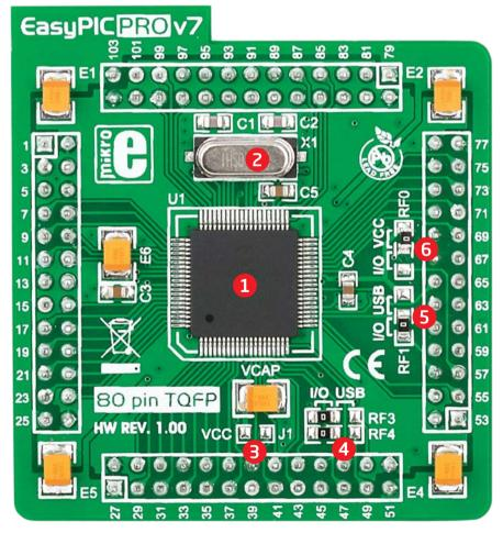
Figure 4-1: Default MCU card with PIC18F87K22
