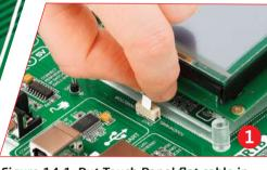
Figure 14-1: Put Touch Panel flat cable in the connector
