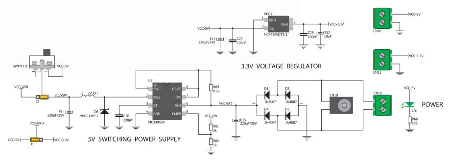
Figure 3-2: Dual power supply unit schematics
