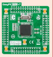
Figure 4-5: Ethernet 80-pin MCU card with PIC18F87J60 microcontroller with internal ethernet module.
