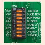
IMPORTANT: In order to use PWM backlight both SW4.1 and SW4.3 switches must be enabled at the same time.
