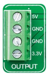
Figure 20-1: Output voltage terminals
