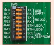
Figure 19-1: Activate SW5.7 and SW5.8 switches to enable pull-up resistors in I<sup>2</sup>C lines of Serial EEPROM.
