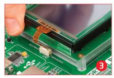
Figure 14-3: Now place GLCD with Touch panel into GLCD socket
