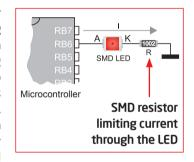
**LED (Light-Emitting Diode)** is a highly efficient electronic light source. When connecting LEDs, it is neccessary to place a current limiting resistor in series so that LEDs are provided with the
