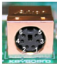
Figure 12.2 - Female PS/2 6-Pin Mini Din Connector at Chameleon PIC socket.
