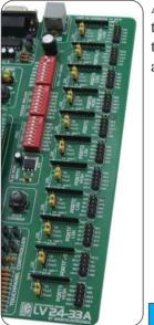
All microcontroller input/output pins can be accessed via IDC10 connectors (2x5) placed along the right side of the board. For each microcontroller port there is one connector providing up to eight port pins and two additional pins connected to VCC and GND.
