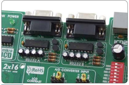
Figure 10 RS-232 communication ports
