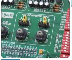
Figure 23 A/D converter test inputs
