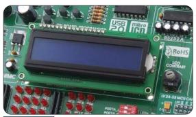
Figure 16 2x16 LCD in 4-bit mode
