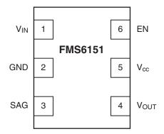
Figure 2. Pin Assignments
