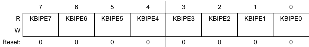
Figure 7-3 KBI Pin Enable Register
