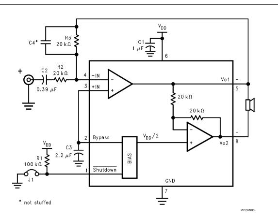
FIGURE 4. REFERENCE DESIGN BOARD SCHEMATIC
