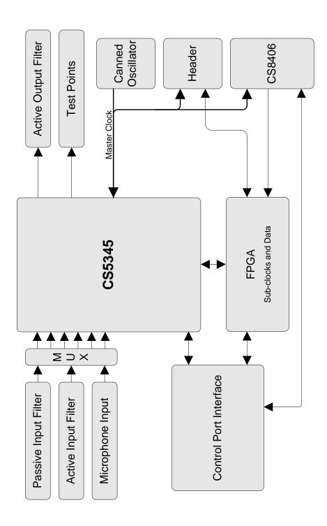
Figure 3. Block Diagram
