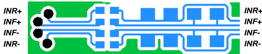
Figure 2. Quad Group Routing of RC Filter Components
