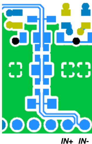
Figure 4. Differential Pair Routing
